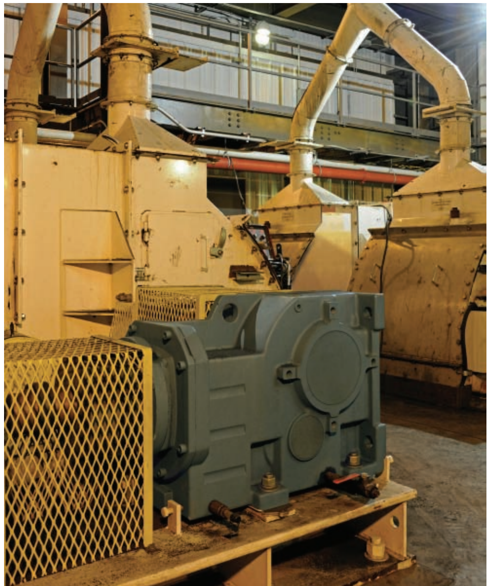
Designed for greater torque density in a compact housing, the Quantis RHB product features a helical-bevel-helical gear train that offers cost-effective, high- and low-speed solutions. Replacing failing gearboxes with the size 168 Quantis units has meant no unplanned downtime at the plant. The maintenance team responsible for keeping coal running reports that since installing the units, it has not had one moment of concern because the units run great with no issues.
